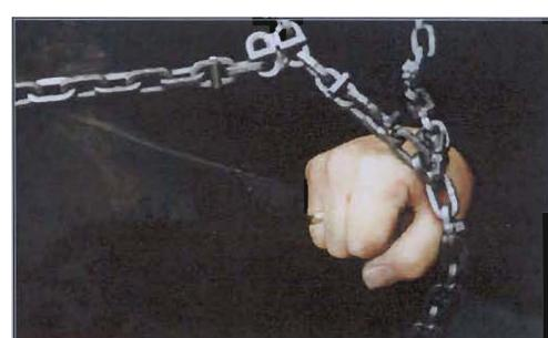
NOTE! Check for correct tension: a fist should fit between the side chain and the tire.
