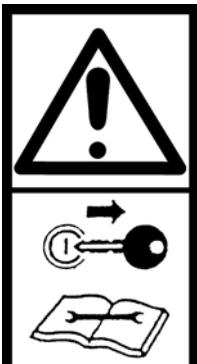
Turn off the engine and remove the key before starting maintenance or repair (located on the top surface of the body).
