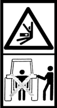
Do not stand near the tie rods of the hydraulic lift when controlling the hydraulic lift (located on the top surface of the lower boom hook).
