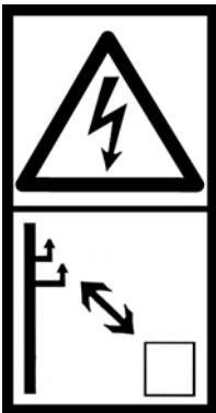
Keep a safe distance from power lines (located on the top surface of the body).
