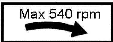
The sign informing about the maximum speed and direction of rotation of the drive shaft. Placed on the PTO guard.
