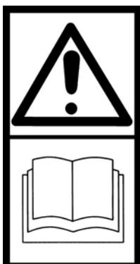
The sign informing about the necessity to familiarize with the instruction manual (located at right side on the top body surface).
