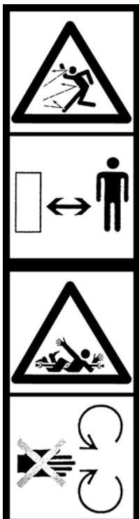
The danger for persons staying within range of snow blower working (located on the rear walls of ejector shield).
