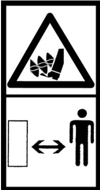
Keep a safe distance from the rotating snow blower rotor (located at the right side of the rotor guard).
