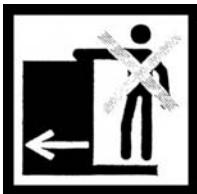
Climbing onto the snow blower while working is prohibited (located on the top surface of the body).
