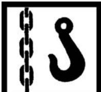
Sign informing about the locations used for lifting machine by lifting devices (located on the top surface of the body in mounting handles).
