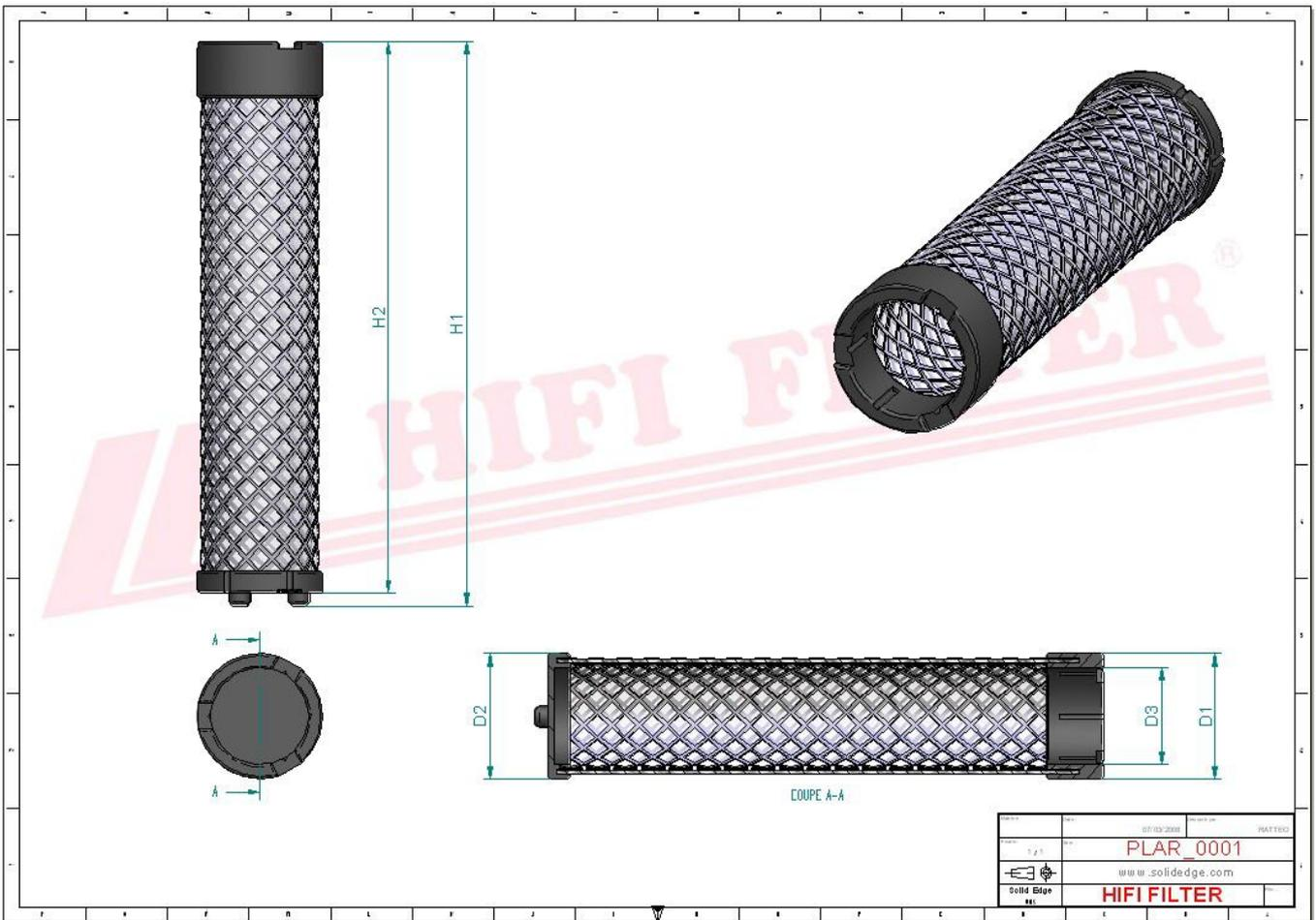
AIR FILTER - RADIAL TYPE - INTERNAL
